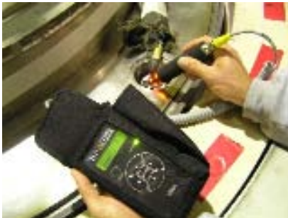
Figure 2: Hydrogen specific leak detection (left) during welding process (right)
